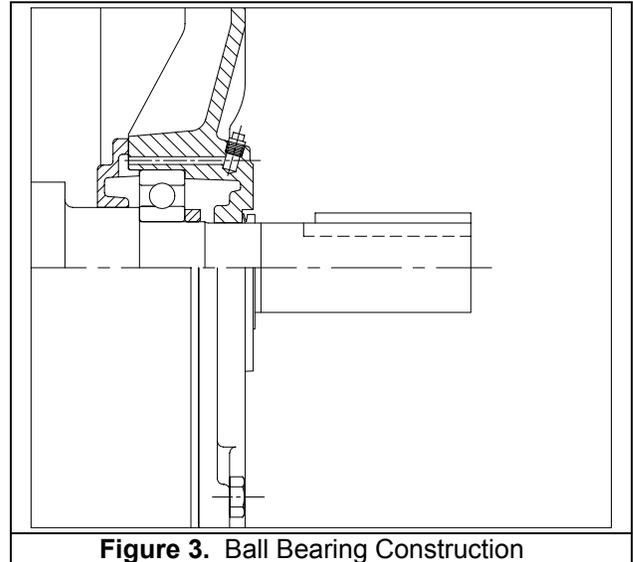
Figure 3. Ball Bearing Construction
